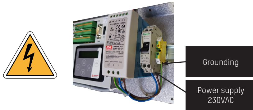
Fig. 30 - Electrical Connections (TRS PMR manual)
