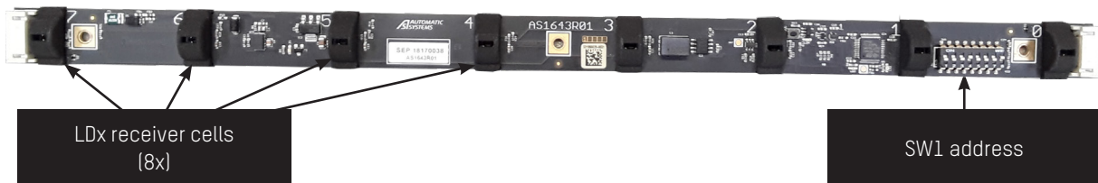
Fig. 105 - Assignment of components: AS1643 circuit board
