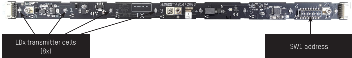
Fig. 103 - Assignment of components: AS1642 circuit board
